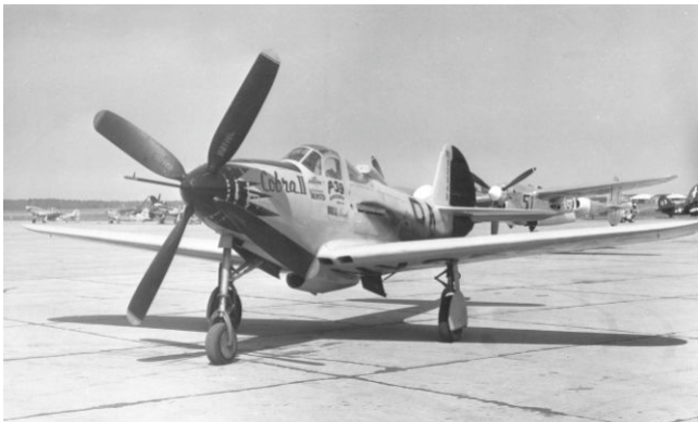
Photo of Cobra II showing shape and position of the underside cooling system An additional cooling system was added to the underside of the fuselage that consisted of a P-40 oil cooler in a streamlined fairing. The pitot tube was re-located to the cannon port in the center of the
