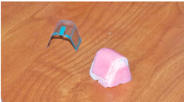
The resin plug and the finished vac-u-form canopy. Photo by Rich Van Zandt form thin and crystal clear replacement canopies that can be posed in the open position.
